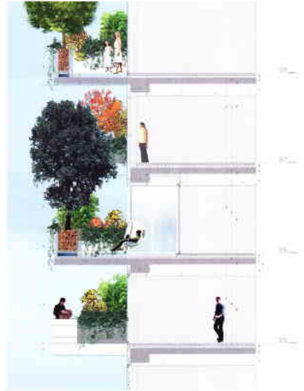
Vertical section of the residential tower Porta Nuova Isola with its vertical forest (Bosco Verticale) in the centre of Milan. © Boeri Studio
